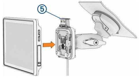
9 Push down the lock (5) to secure the device to the mount.
