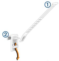
2 Connect the rubber strap to the back of the mount 3.
