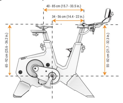
Before you assemble the Tacx NEO Bike Plus trainer, consider that the saddle and handlebar have set screws installed from the factory that can be adjusted and tightened using a hex key. To install the 4 handles as shown in this manual, you must remove the 4 set screws using a hex key.
