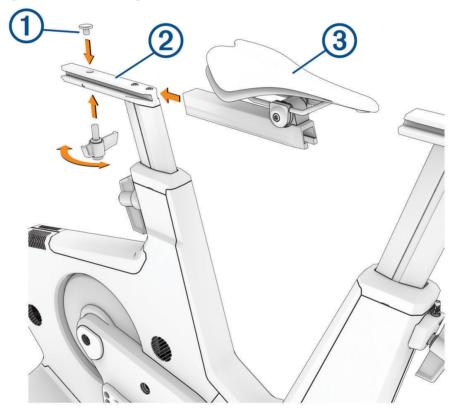
4 Slide the saddle 3 onto the saddle rail.
