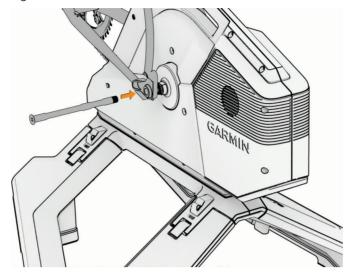
**11** Tighten the axle to the torque specification indicated on the axle or in your bike instructions.
