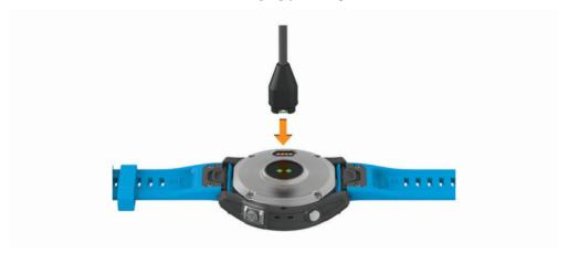
2 Plug the large end of the USB cable into a USB charging port. The watch displays the current battery charge level.
