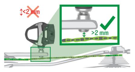
9 If the pedal rubs the chain, add one washer (included) between the spindle and the crank arm to increase clearance.
