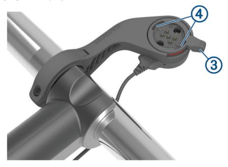
7 Align the tabs on the back of the Edge device with the eBike mount notches 4.
