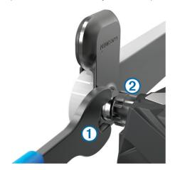
**NOTE:** The right pedal has a left-handed (reverse) thread. As you unscrew the pedal, the pedal pod cable disengages from the spindle.
