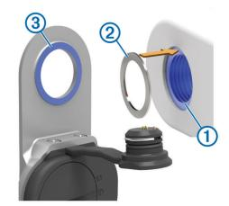
Make sure the pedal pod mounting face ③ contacts the crank arm only at its mounting face (or the washer used to fill the recess).
