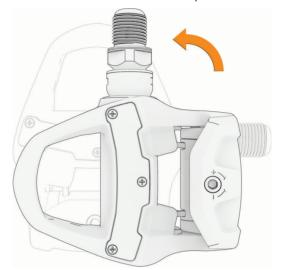
5 Turn the pedal 90 degrees, and hold it with the threaded end to the side for 2 seconds.
