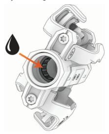
Apply a thin layer of grease to the highlighted areas of the new spindle.NOTE: You should apply enough grease to fill the groove on the rubber seal 3.
