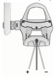
• For the Rally XC pedal bodies, use a 3 mm hex key to adjust the release tension screw equally on both sides of the pedal.
