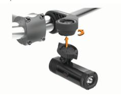
**12** Adjust the headlight angle so it is parallel to the road, and use the 4 mm hex key to tighten the screw.
