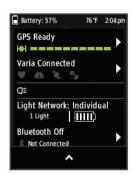
The connections screen appears. A flashing icon means the device is searching.
