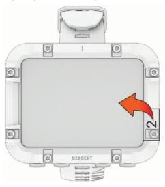
8 Slide the applicator card across the screen protector to remove air bubbles and firmly adhere it to the dive computer screen.
