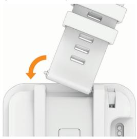
**NOTE:** Make sure the band is secure. The pin should align with the holes on the dive computer.
